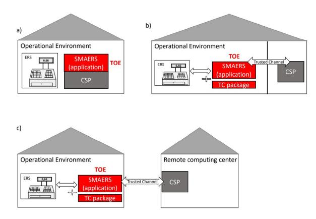
Figure 2. The TOE is always operated as local component. a) Platform architecture b) client-server architecture with local computing center c) client-server architecture with remote computing center
