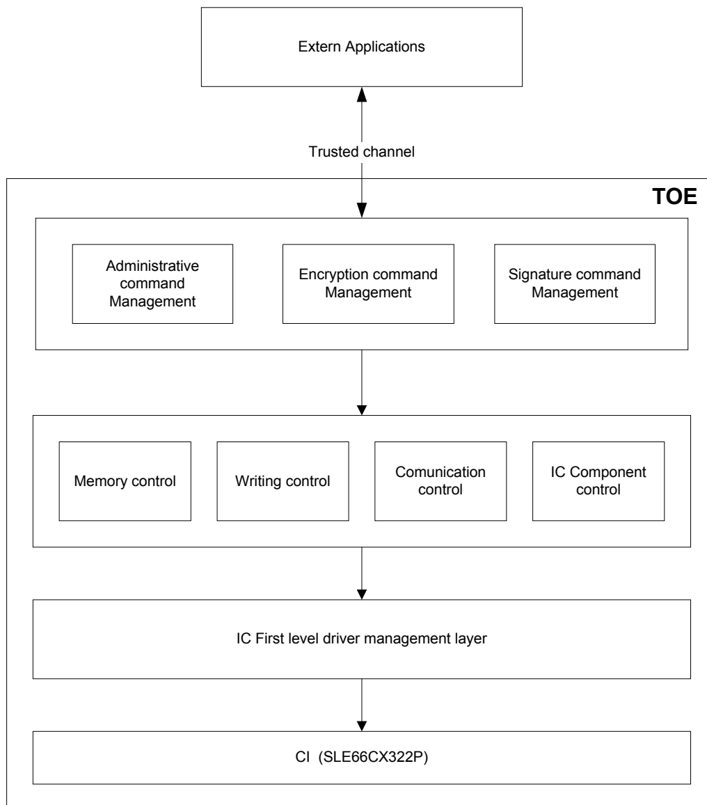
Figure 2-1: TOE layer description
