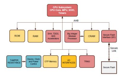
Figure 1 TOE Architecture
