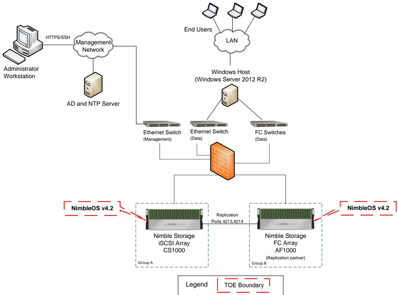
**Figure 3 – Evaluated Configuration of the TOE**
