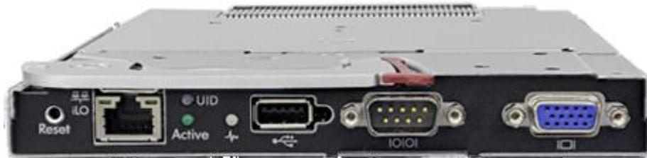
**Figure 2 – HP BladeSystem OA Module (Example)**
