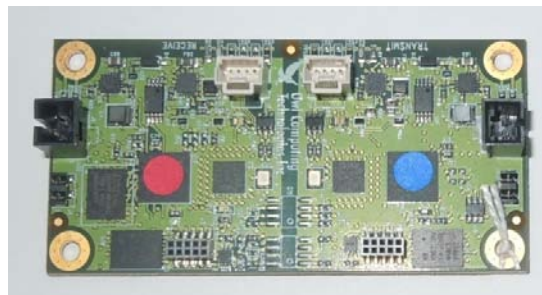
Figure 2 - Owl 010-Rev E DualDiode Communication Card
