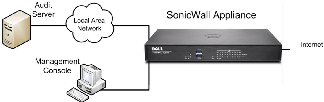
**Figure 1 – TOE Diagram**
