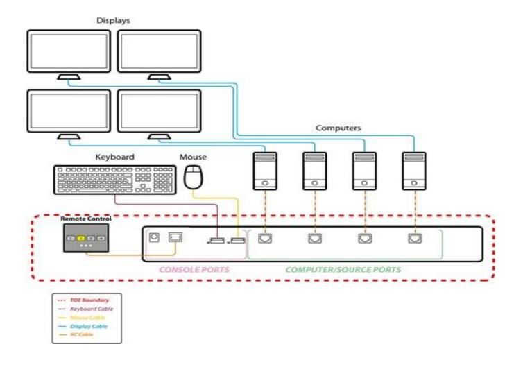
Figure 2: TOE Architecture (Filter)
