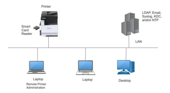
**Figure 1 - Representative TOE Deployment**
