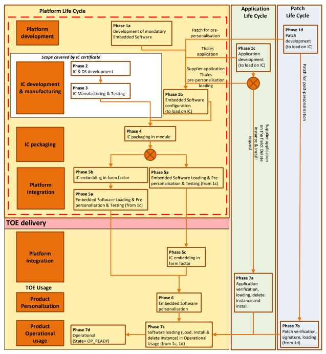
Figure 2: Manufacturing phases description
