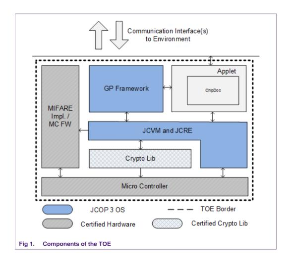
The TOE consists of an applet which is executed by a software stack that is stored on a Micro Controller. For a complete picture of the TOE see Fig 1, and for details with regards to the different components see section 1.3.1. The TOE is delivered in closed configuration, meaning that all other interfaces apart from the SSCD ones are locked and do not act as communication interfaces towards the environment.
