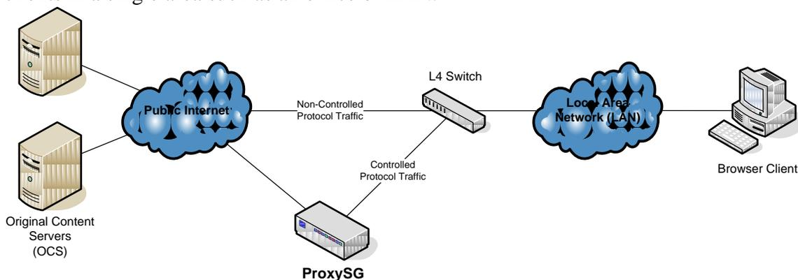
**Figure 2 – Transparent Forward (Gateway) Proxy Deployment**
