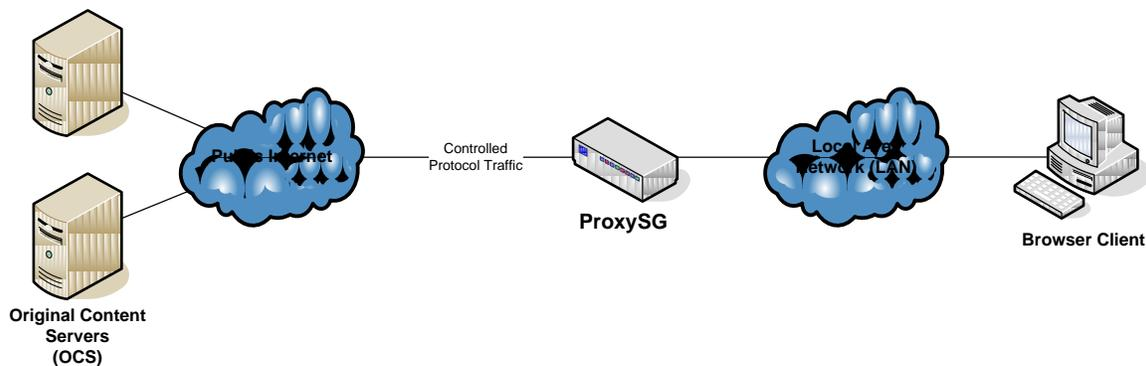
**Figure 3 – Explicit Forward (Gateway) Proxy Deployment**
