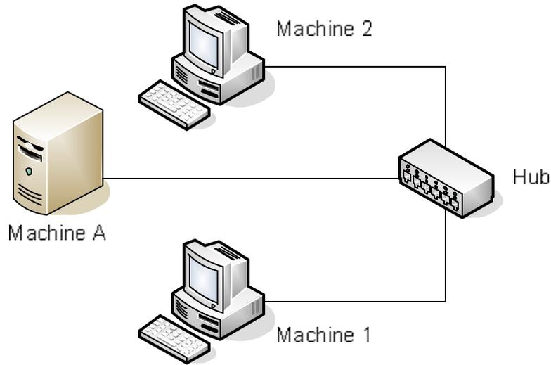
45. Machine A acts as the remote PC running the SafeBoot Administration Server, which consists of SBAdmin, SB Server and the SafeBoot Object Directory. These are connected to the SafeBoot Device Encryption PC client machine over a network using the TCP/IP protocol.
