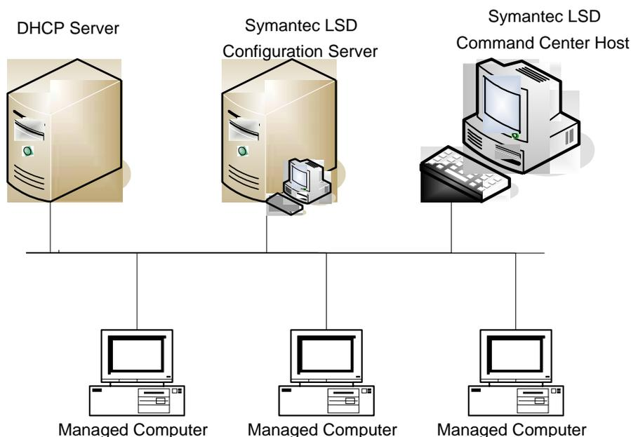
Figure 1-2: Network Environment for the TOE
