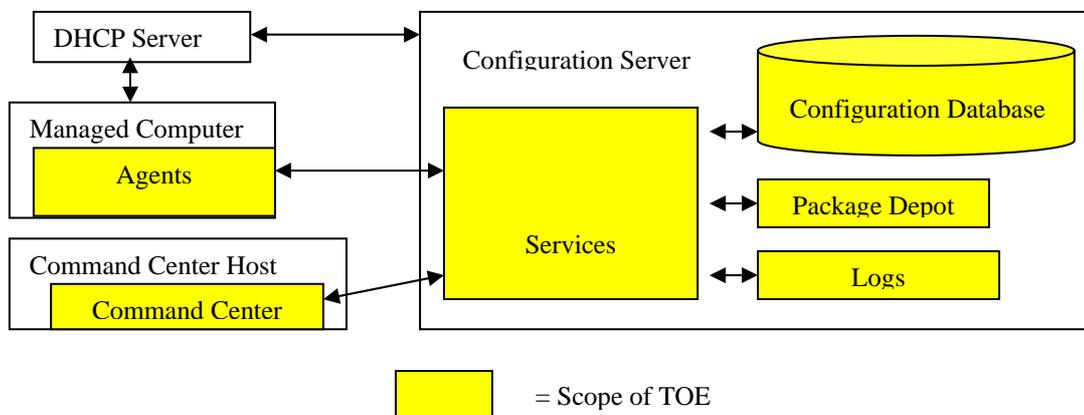
Figure 1-1: Components and Scope of the TOE
