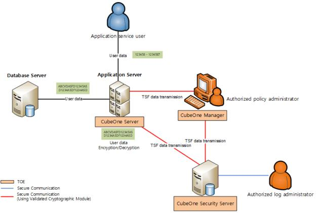
Figure 1. Plug-in type operational environment
