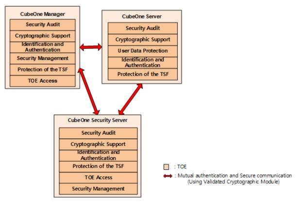
Figure 4. Logical scope of TOE
