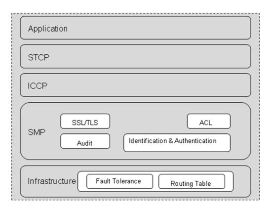
The specific functionality detailed in the white boxes is executed in a distribute way. The modules SSL/TLS, ACL, Audit, Identification & Authentication and Fault tolerance are executed in the OMU board. The modules relating with the routing table and connection filtering out of the management network are executed on the interface board.
