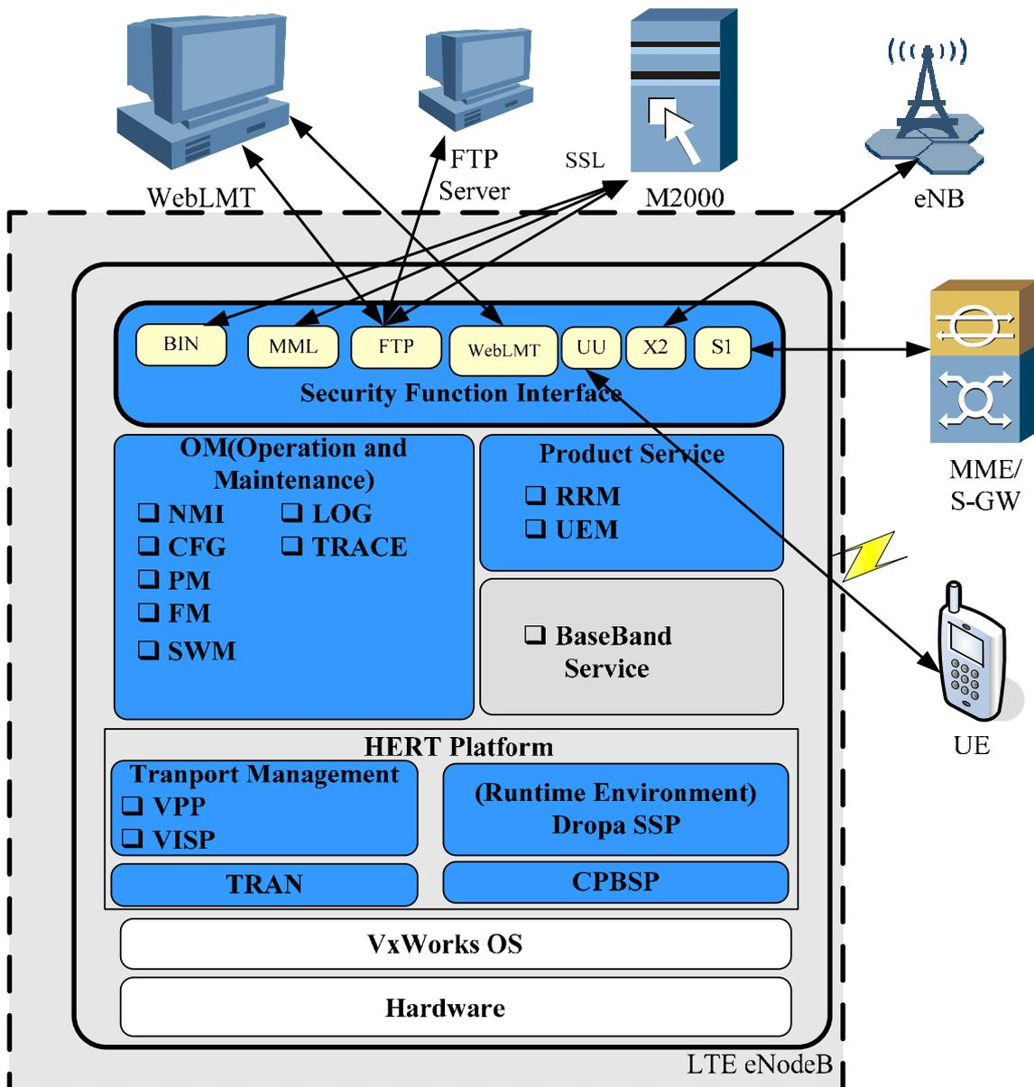
Figure 4 Software architecture
