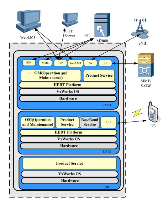
In the above diagrams, the content of the blue areas (excluding the grey boxes) are parts of the TOE. The TOE includes Operation and Maintenance (OM), Product Service, Transport Management, TRAN, CPBSP, Dopra SSP and HERT platform.
