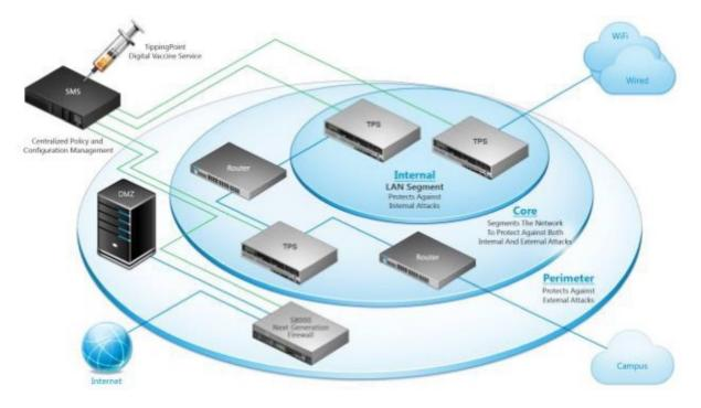
Figure 1 - Sample TPS Network Deployment Scenario
