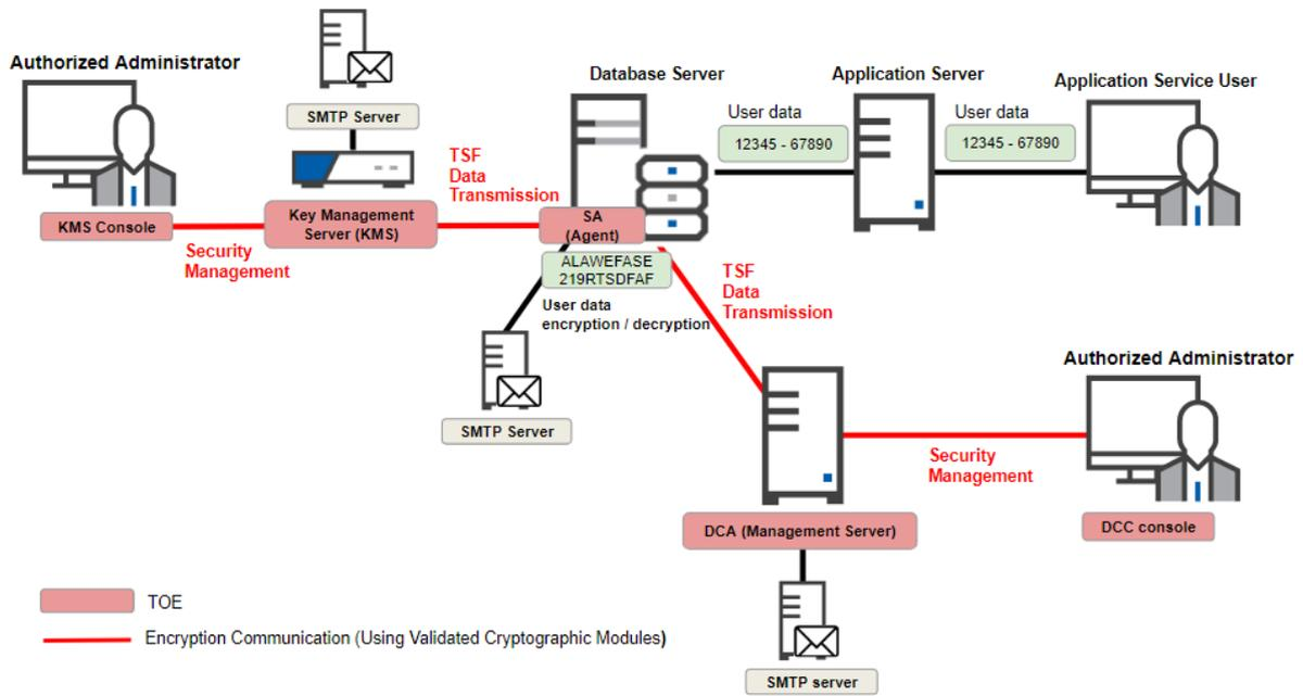
[Figure 1-2] represents the operating environment of 'agent and management server integrated type'. This is installed SA and DCA together in the protected DB, and the DCC Console and KMS are physically separated and installed.
