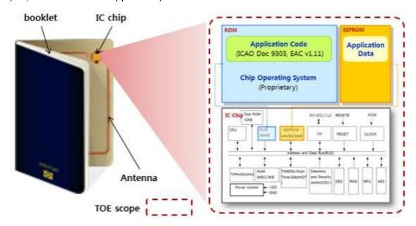
[Figure 2]Physical boundary of the TOE
