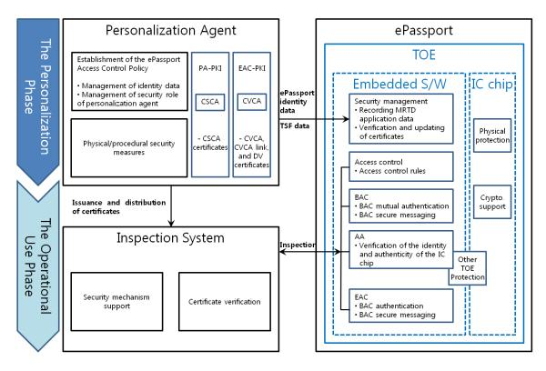
[Figure 1]Operational environment of the TOE
