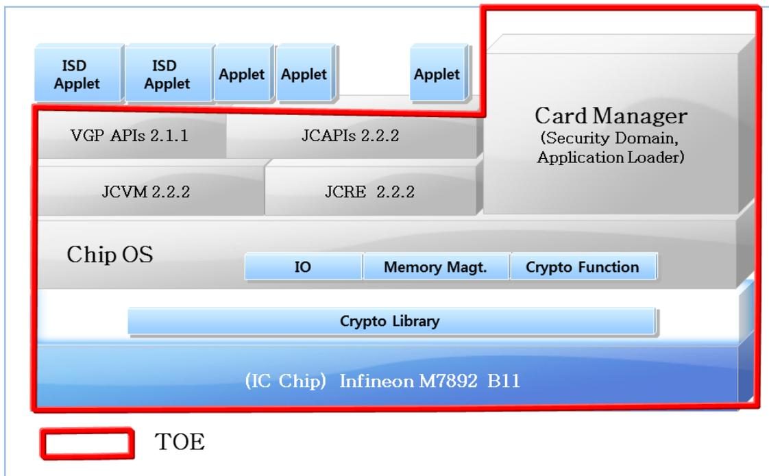
[Figure 2] Architecture of the TOE
