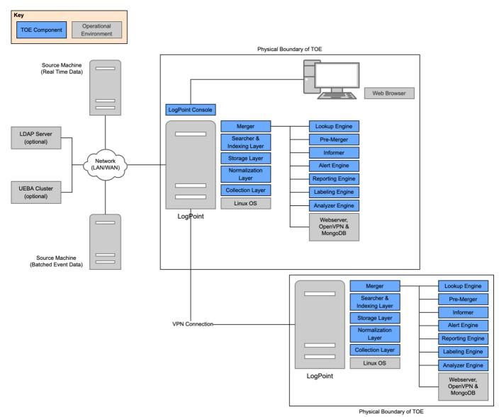
Figure 6 Multiple Appliance LogPoint Deployment
