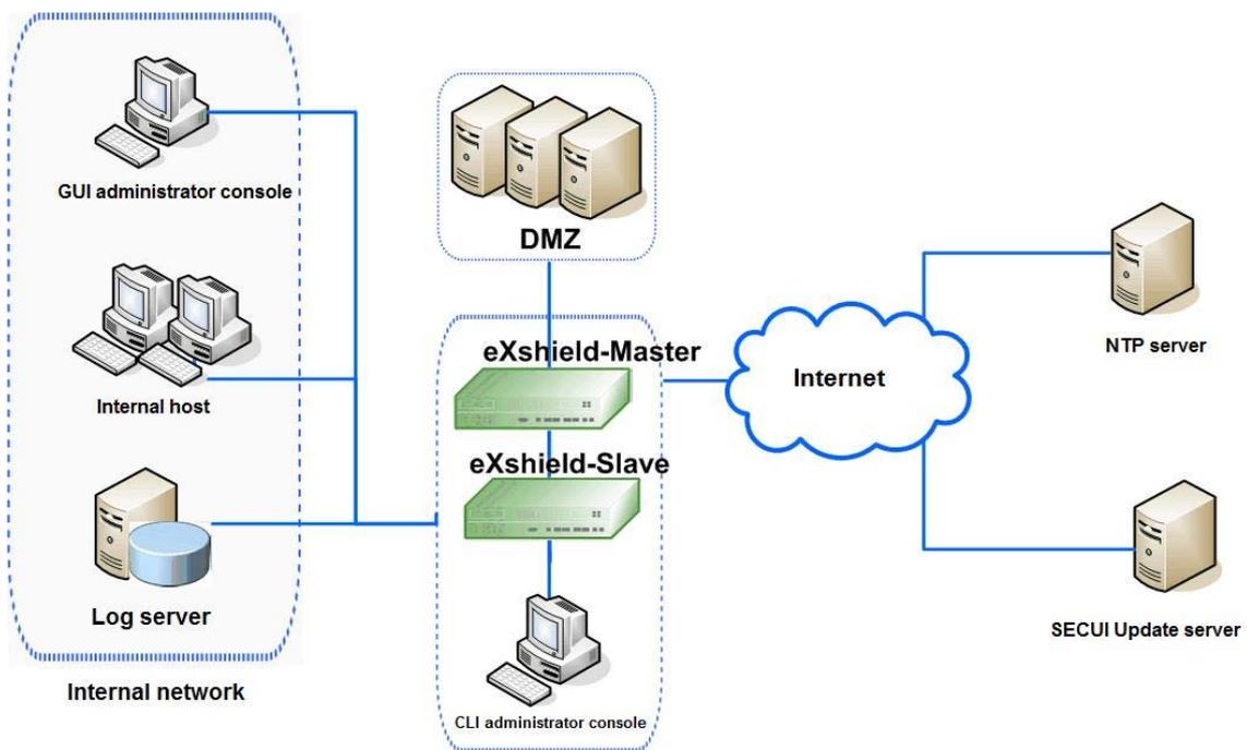
(Figure 2) Configuration of eXshield Security Switch V1.0: 2
