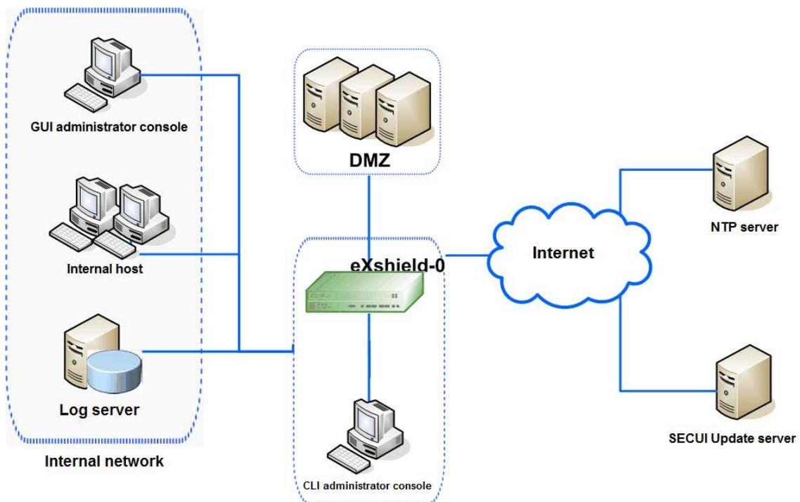
(Figure 1) Configuration of eXshield Security Switch V1.0
