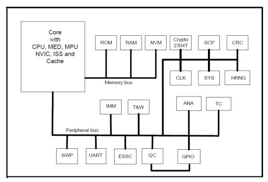
Logically the TOE provides cryptographic support for TDES, AES, and RNG, memory protection unit supporting different memory access levels, authentication of the smartcard IC, support for loading of flash content in secured locations and in loading by authorized users only. In addition, optional software libraries with HW NVM support and cryptographic support for TDES AES, RSA, ECC, SHA, Hash and MAC calculation and RNG is also included.
