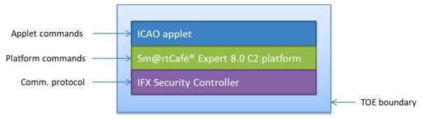
The TOE is an applet named ePass applet based on Sm@rtCafé® Expert 8.0 C2 platform, which is used as an ICAO eMRTD, which can be configured to support the different authentication mechanisms.
