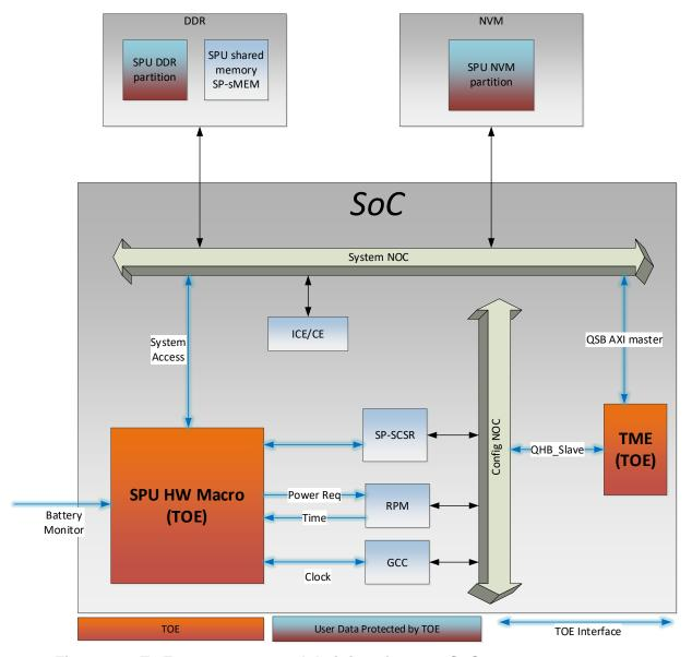
Figure 3-1 TOE components and their interfaces to SoC
