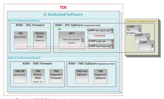
Figure 3-2 TOE IC dedicated software components
