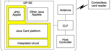
The TOE is a Java Card system that provides a secure signature creation device (SSCD) with key generation for creating an electronic signature and authenticating users. The TOE is embedded as a secure element (eSE) on the mobile phone.
