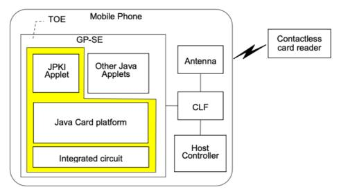
The TOE is a Java Card system that provides a secure signature creation device (SSCD) with key generation for creating an electronic signature and authenticating users. The TOE is embedded as a secure element (eSE) on the mobile phone.
