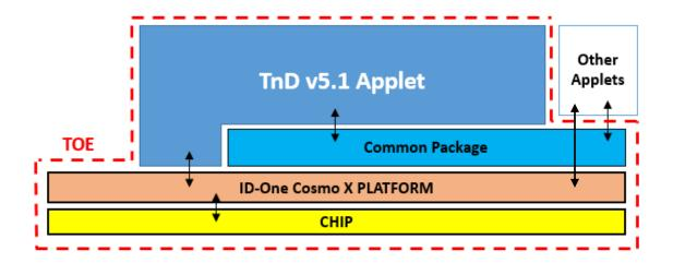
Figure 2 TOE's logical architecture
