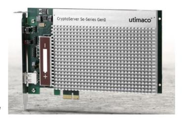
To enable communication of the cryptographic module with a host, the PCIe security module offers a PCIe interface and two USB interfaces. The PCIe security module is plugged into the PCIe bus interface of the backplane.
