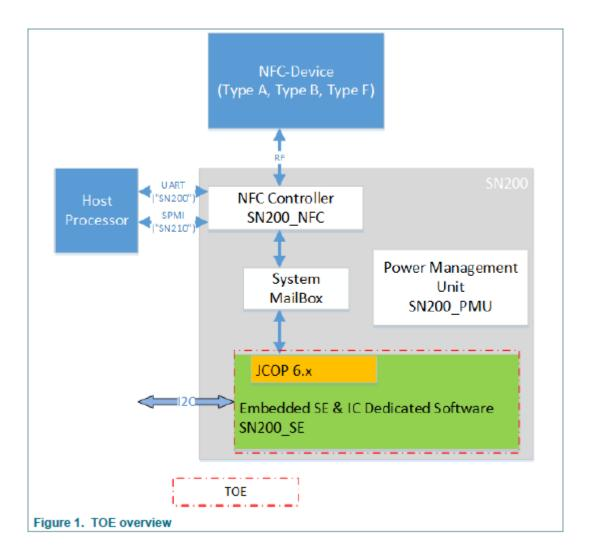
The TOE directly supports an I2C communication interface and communicates with the integrated NFC controller via the System Mailbox. The integrated NFC controller is not in scope of this evaluation, however, provides up to 4 gates for external users to communicate with the TOE supporting Card Emulation Mode Type A, Type B and Type F as well as a wired Interface using APDUCard Gate. Extended length APDU communication is supported for Card Emulation and wired mode, up to 32kBytes.
