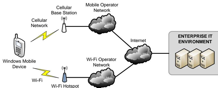
**Figure 2 - Device Connectivity**
