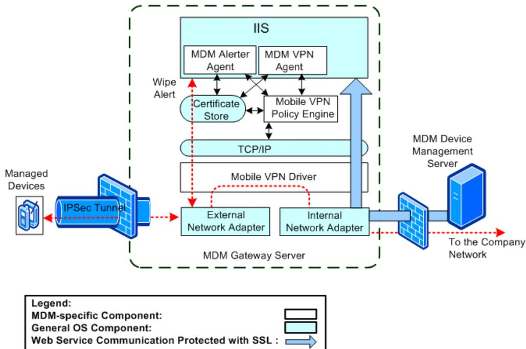
**Figure 3 – Components of the MDM Gateway Server**
