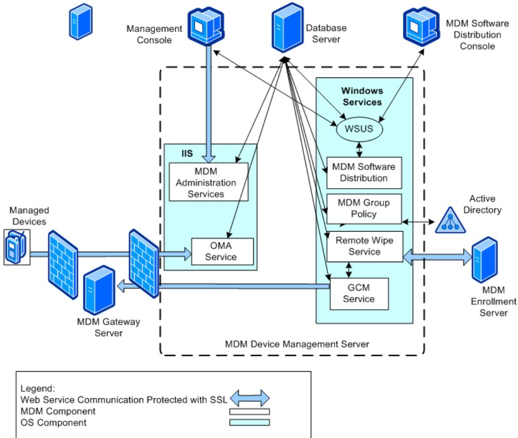
Figure 5 – Components of the MDM Device Management Server
