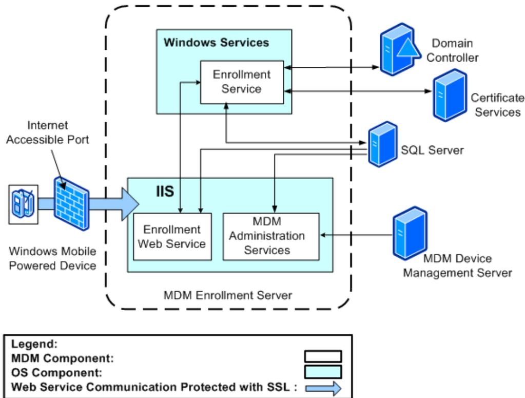
Figure 4 – Components of the MDM Enrollment Server
