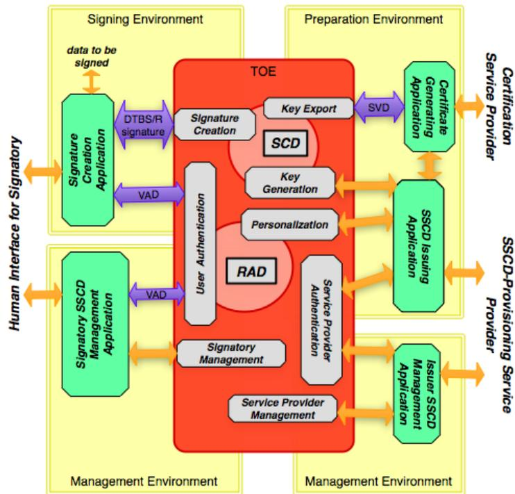
**Figure 2: TOE and Operational environments with Key Generation**
