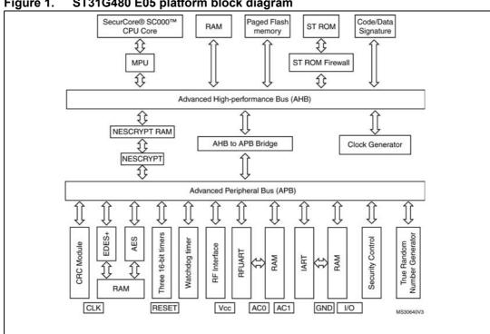
Figure 1. ST31G480 E05 platform block diagram
