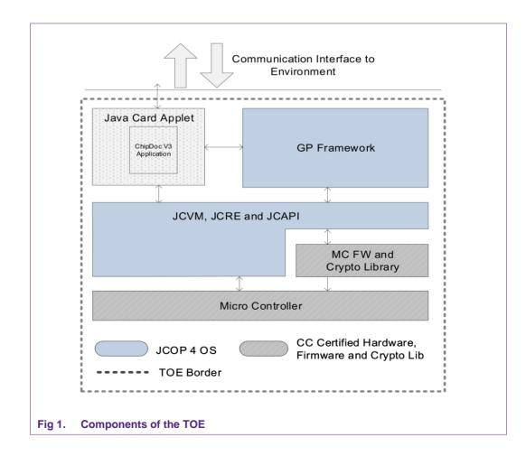
The TOE consists of an applet which is executed by a software stack that is stored on a Micro Controller. For a complete picture of the TOE see Figure 1, and for details with regards to the different components see section 1.3.1.
