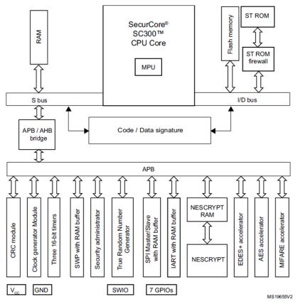
The ST33HTPH hardware supports an SPI interface compliant with [PTP 1.05] for integration with controllers and system drivers.
