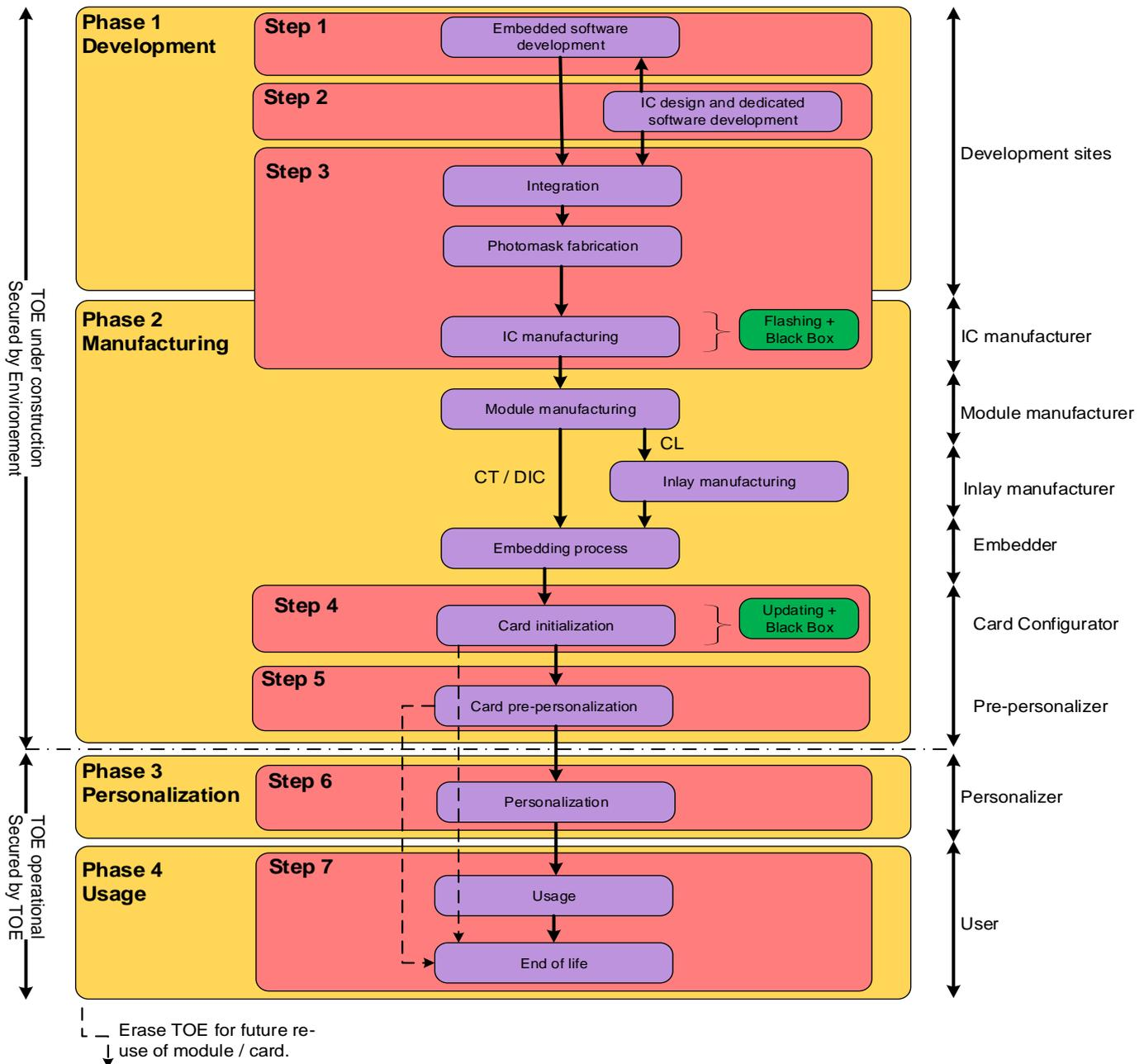
**Figure 5 Flashing and dedicated BlackBox loading at IDEMIA factory on card; pre-personalization on card**
