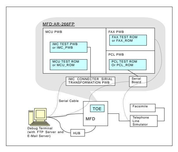
Figure 2-2 Configuration of Evaluator Testing
