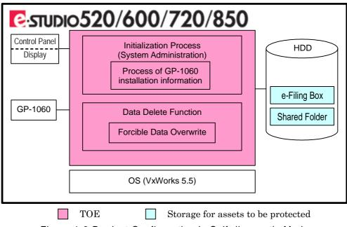
Figure 1-3 Product Configuration in Self-diagnostic Mode
