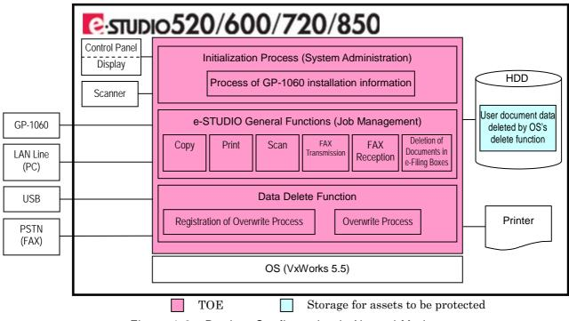
Figure 1-2 Product Configuration in Normal Mode
