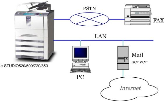
Figure 1-1 Typical operating environment of the TOE
