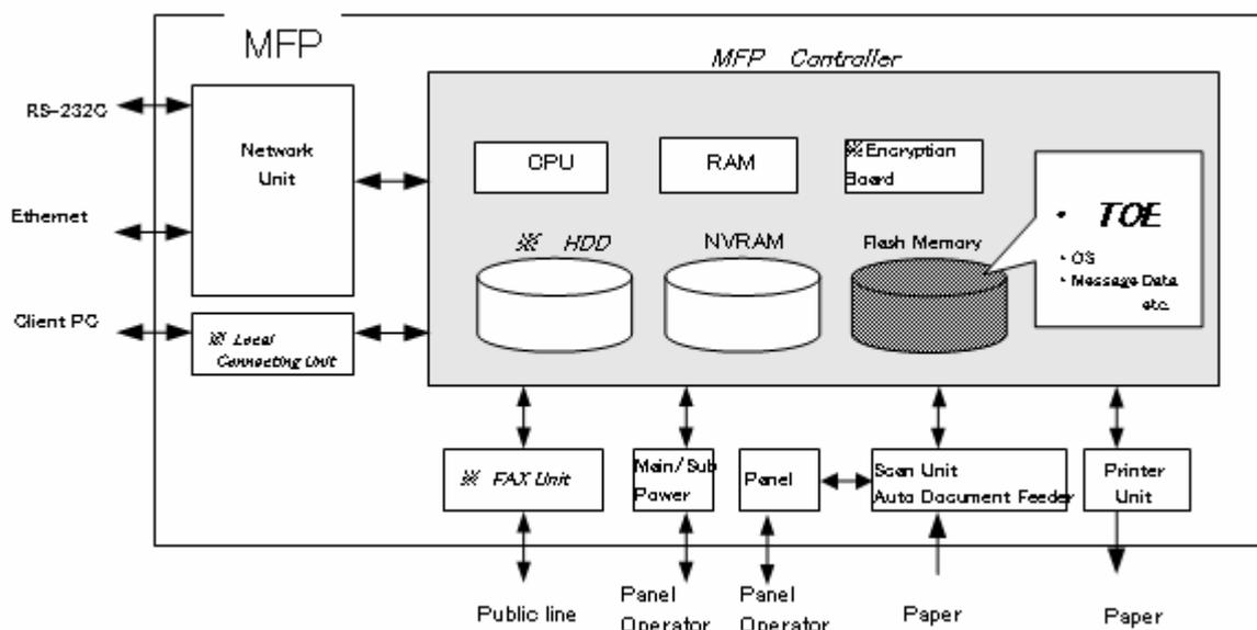
**Figure 1-1: Hardware structure that relates to TOE**
