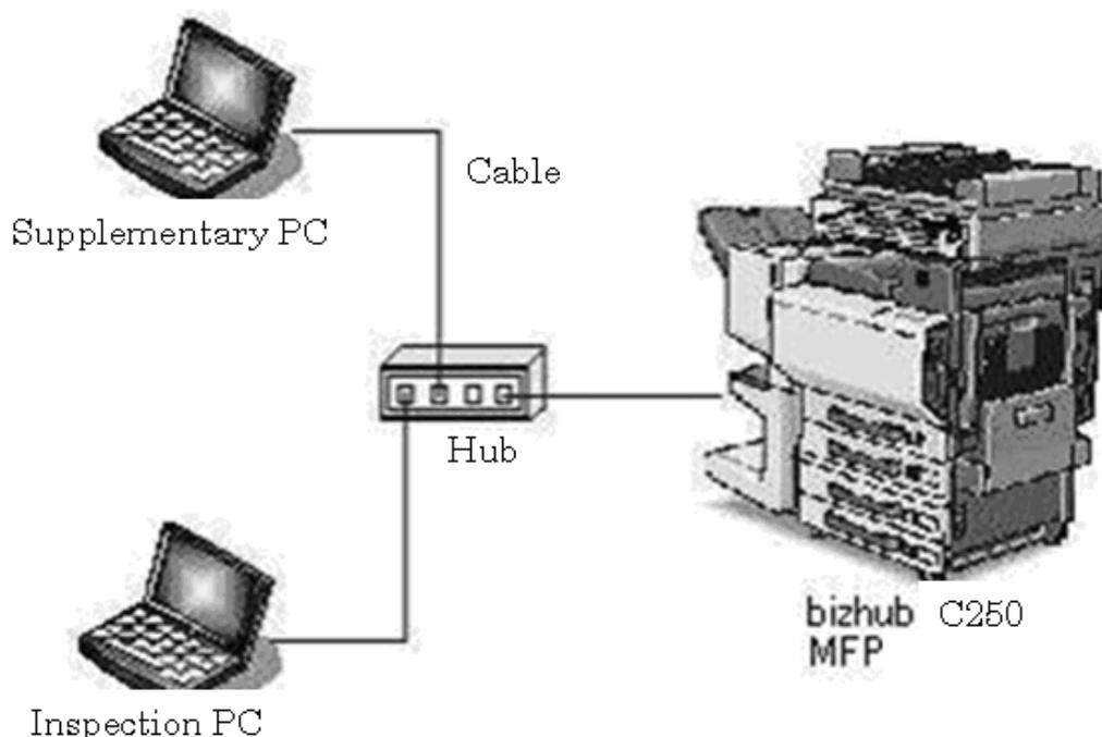
Figure 2-2: Evaluator test (Intrusion test) configuration
