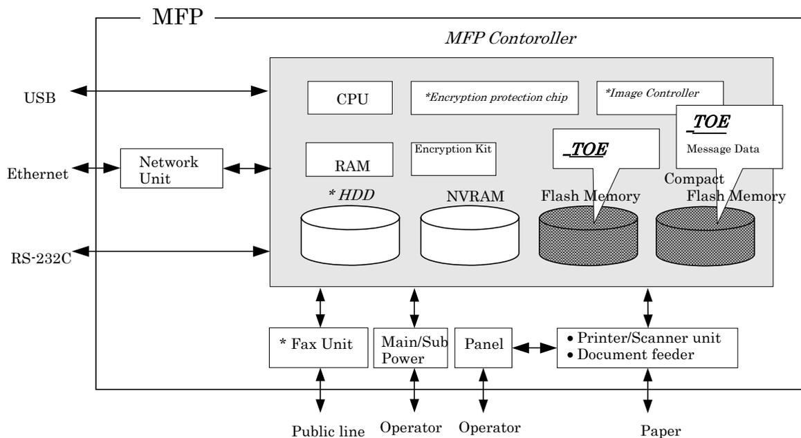
**Figure 2 Hardware composition that relates to TOE**
