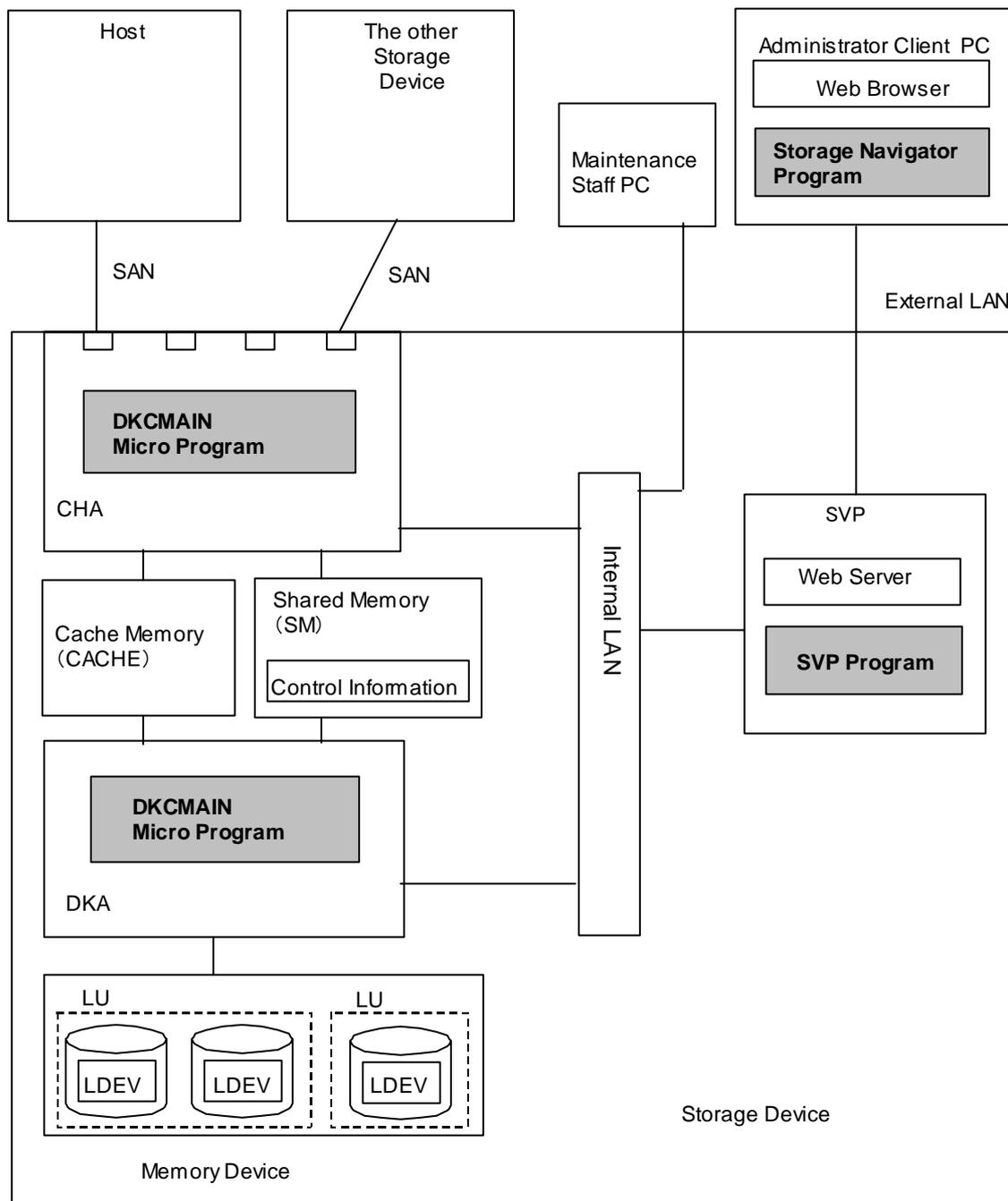
Figure 2.2 Storage Device Configuration
