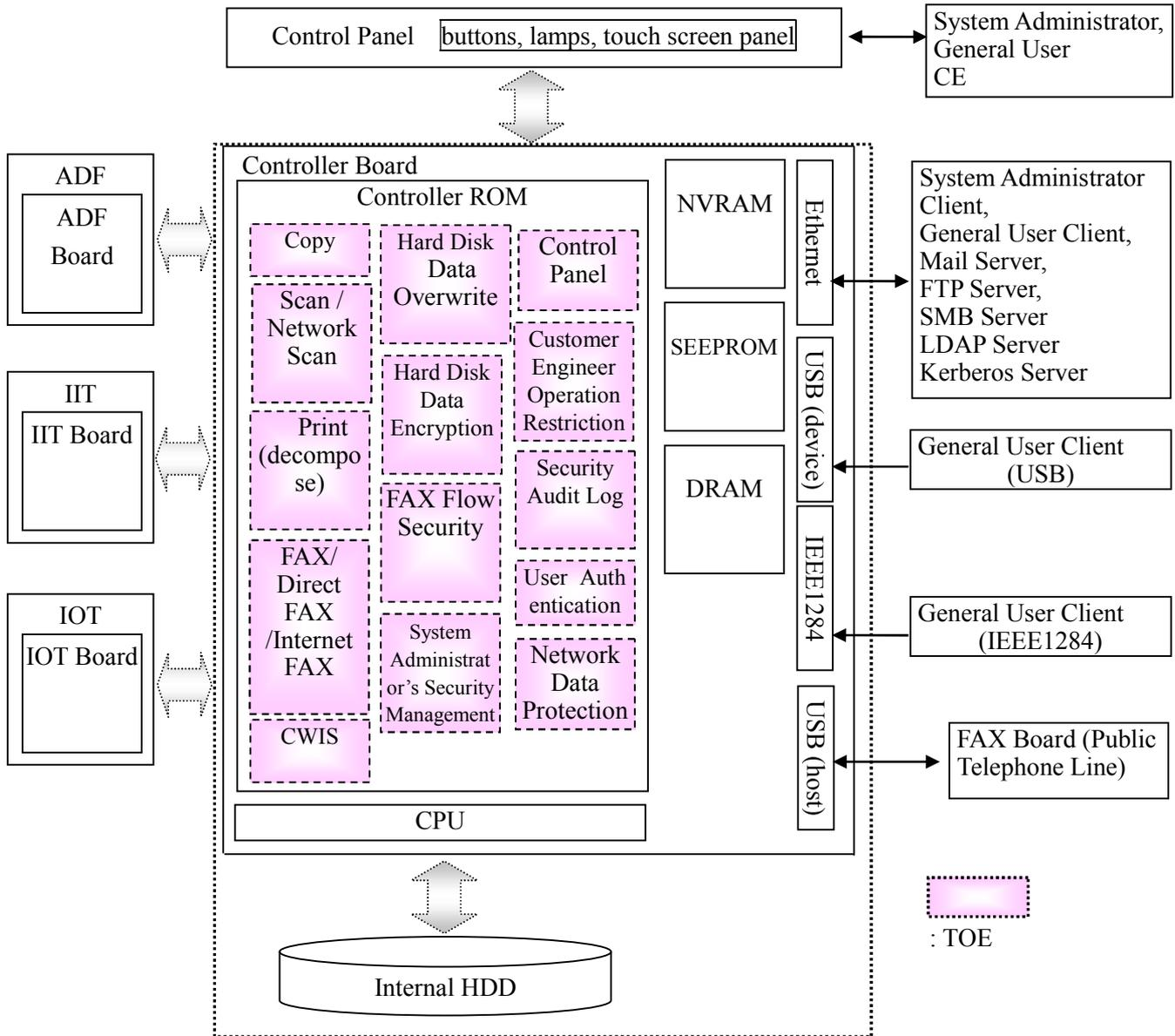
Figure 4: MFD Units and TOE Physical Scope
