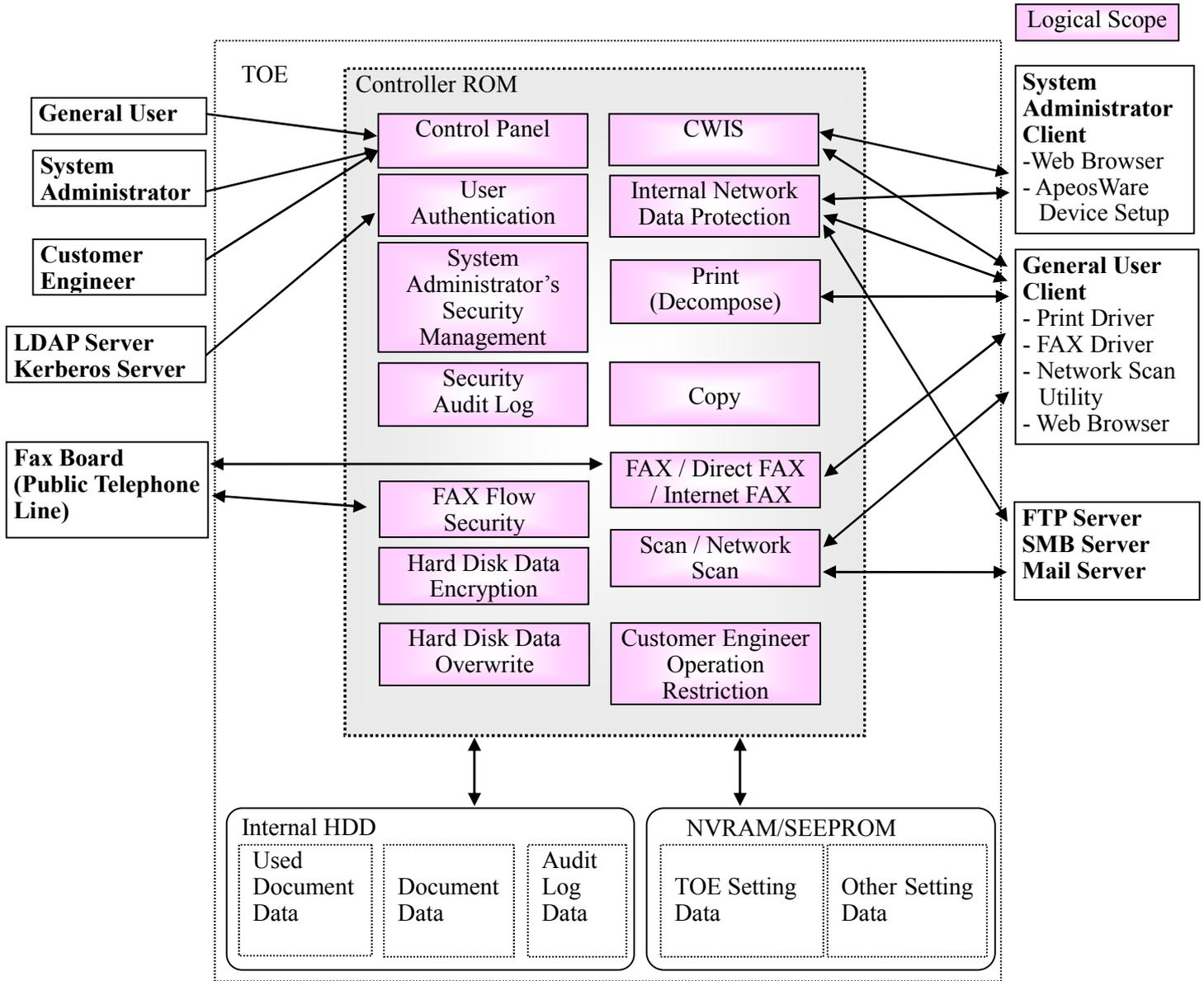
Figure 2: MFD Units and TOE Logical Scope
