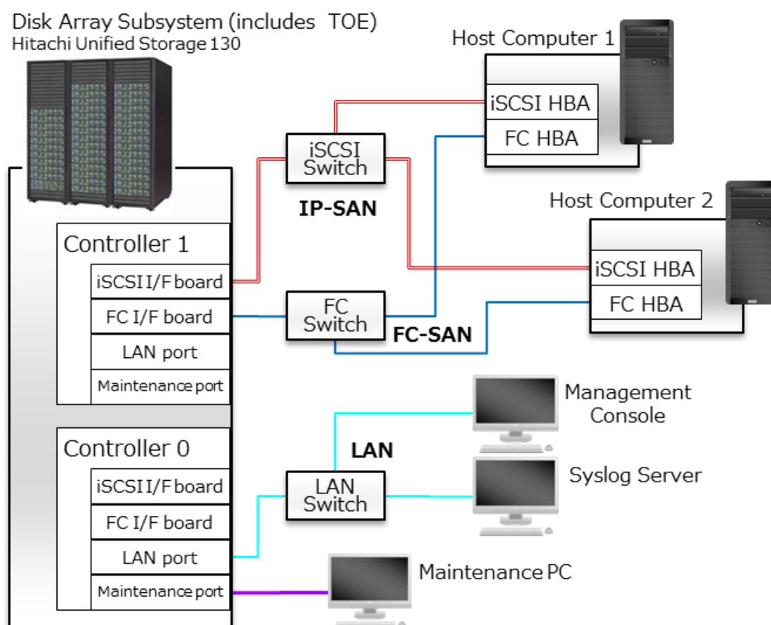
Figure 7-1 Configuration of the Developer Testing
