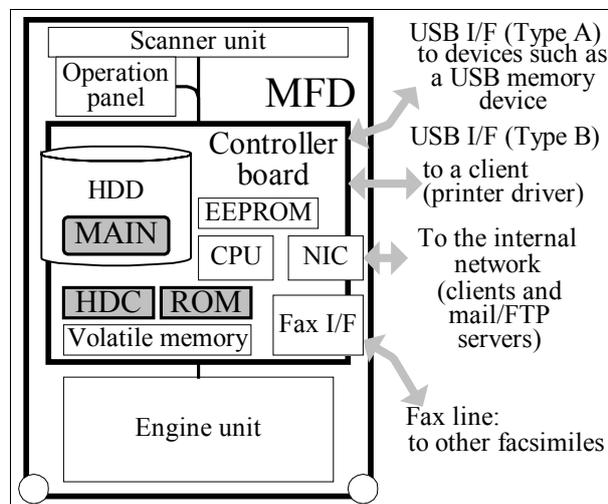
Figure 2: TOE and physical configuration of the MFD
