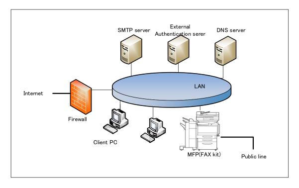
Figure 4-1 Operational environment of the TOE
