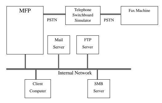
Figure 7-1 Configuration of the Developer Testing
