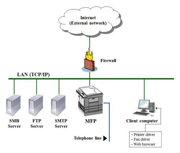
Figure 4-1 Operational Environment of the TOE
