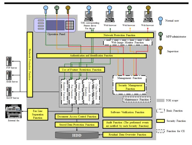
Figure 3: Logical Scope of the TOE
