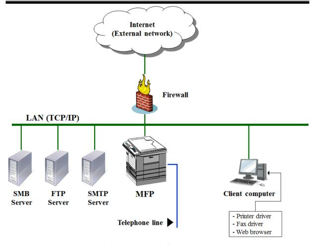
Figure 1: Example of TOE Environment
