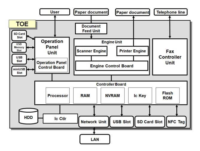
Figure 2: Hardware Configuration of the TOE
