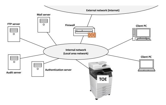
Figure 4-1 Operational Environment of the TOE
